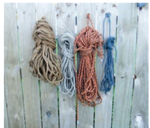
From left Hemp rope used in early mountaineering, early nylon rope, present day Kernmantel rope and present day guiding short rope.
